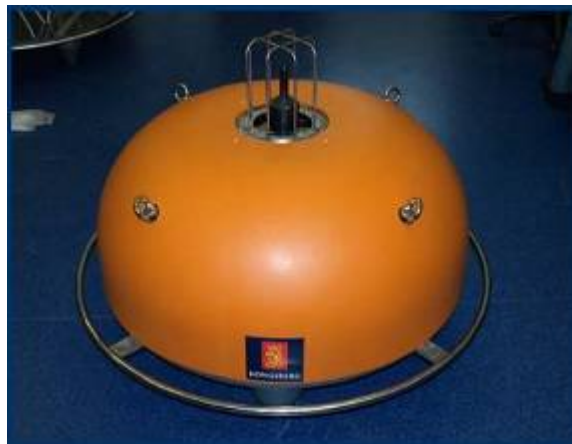
Figure 6. The Remote Undersea Noise Evaluation System (RUNES).
