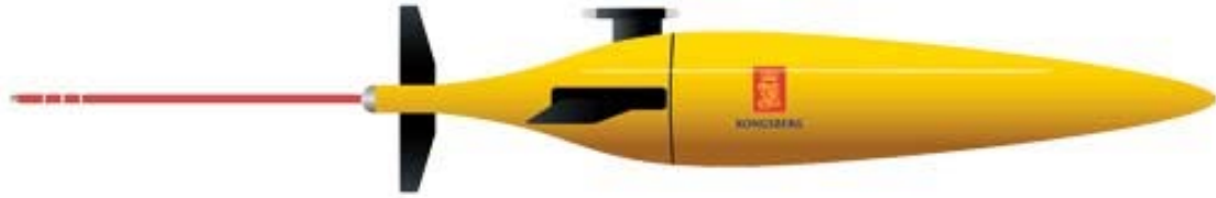
Figure 10. Seaglider – The PAM module is fitted in the rear instrument section and the hydrophone is adjacent to one of the dorsal fins
