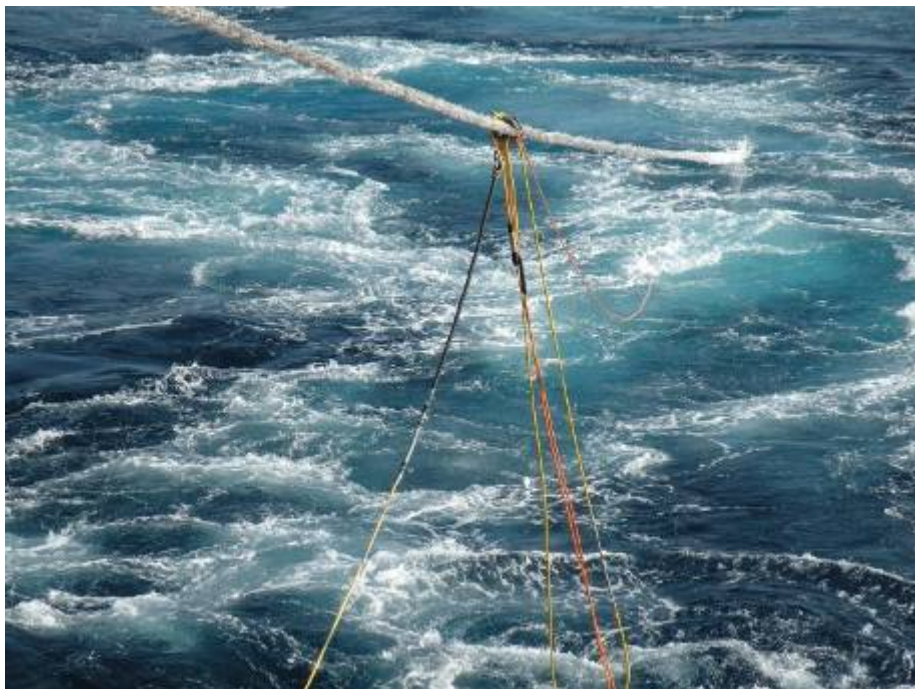
Figure 1. PAM towed array entanglement with lead-in
